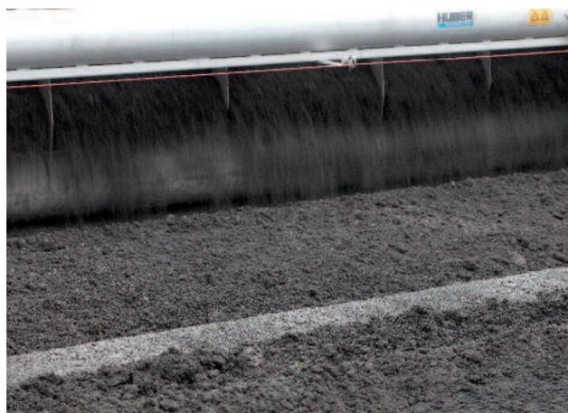
*Backmixing and aeration of sludge*
