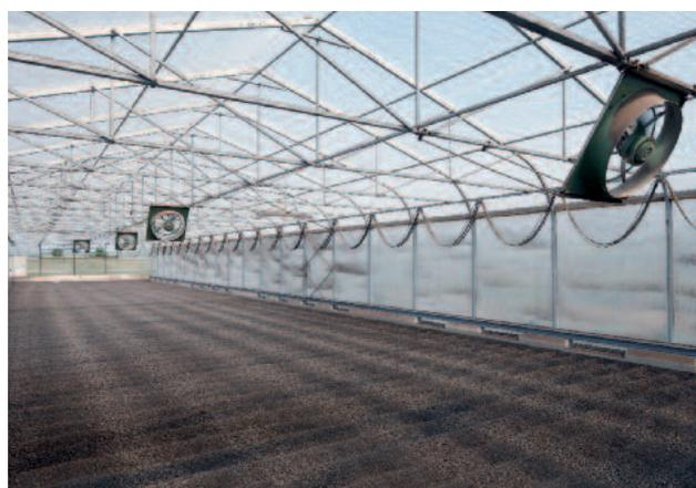
*Ventilators blow dry air over the sludge bed.*
