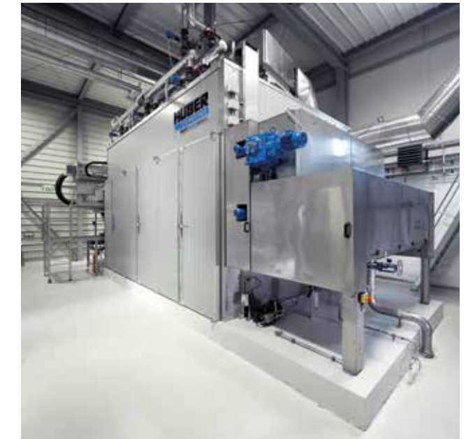
Head piece with integrated automatic belt cleaning.
