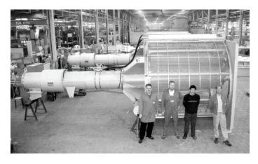
treatment plant is designed for the maximum storm weather flow of 4500 l/s. This flow can be handled by two HUBER ROTAMAT Wedge Section Screens Ro 2 3000 x 6 mm. One screen is installed as a standby unit..
