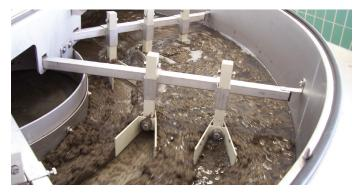
The thickened sludge is stored in a fully mixed short span retention tank and then is dosed with a polymer and is dewatered in a HUBER QPRESS.
