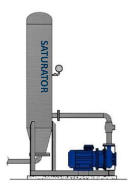
A recycle stream of treated effluent is taken from the discharge end of the HyDAF and is pressurised to 450 kPa.
