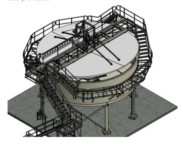
The sludge rake operates by pushing lime solids along the bottom of the tank using 10 GR316 SS blades with neoprene squeegees.
