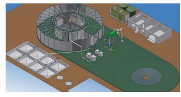
To facilitate site installation the entire structure of the activated sludge process was fabricated using the Roadtrain® bolted design.
