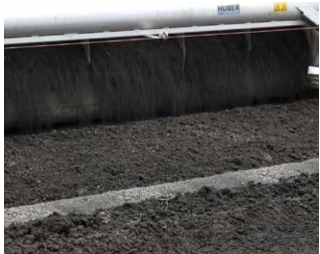
The HUBER Sludge Turner SOLSTICE® ensures an optimal drying bed – the sludge is spread, granulated, aerated, turned and backmixed.
